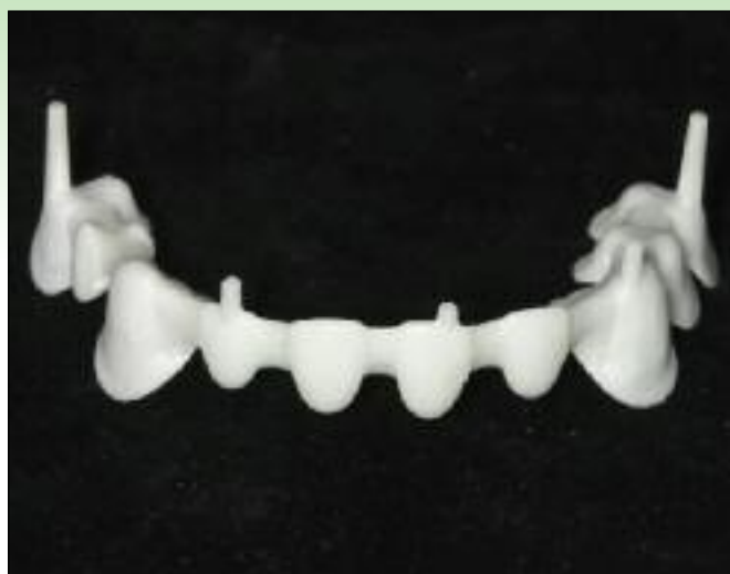
Milled frame following 12 hours of "hard sintering".
