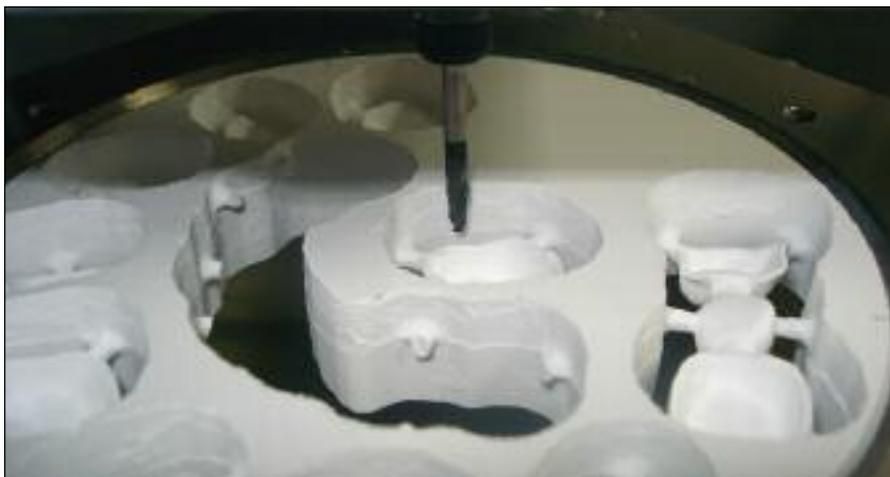
Figure 4. Milling head.
